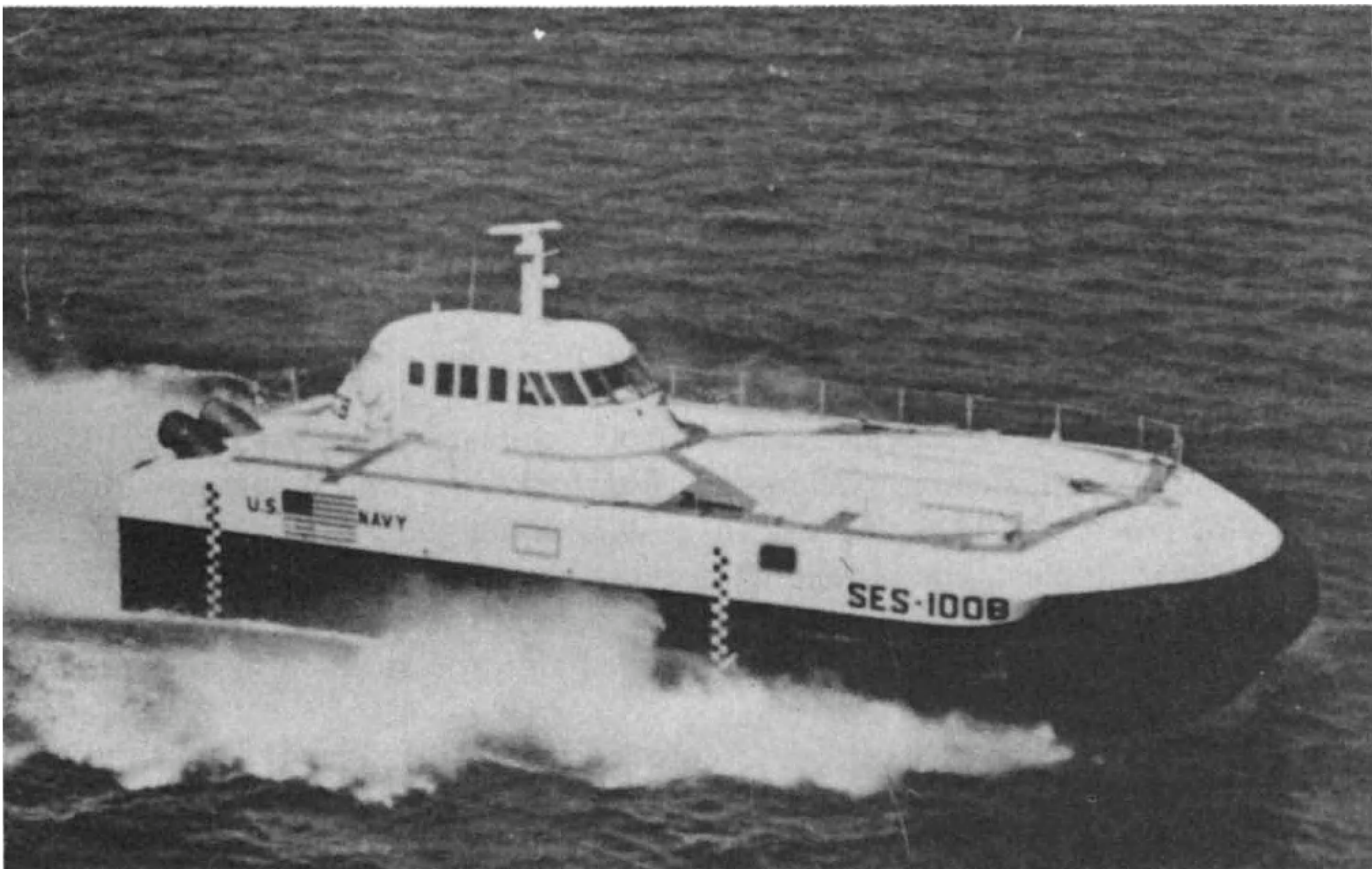
FIG. 1.5. Surface effect ship-SES 100. (101) This photograph shows SES 100, a 100-ton surface effect ship completed in 1975 by the Bell Aerospace for the U.S. Navy. This ship cruises at a speed of over 80 knots. The U.S. Navy plans to build surface effect ships as large as 2000 tons with a cruising speed of 100 knots.
