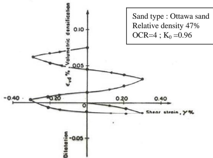
Figure 5. Volumetric strains under cyclic loading
