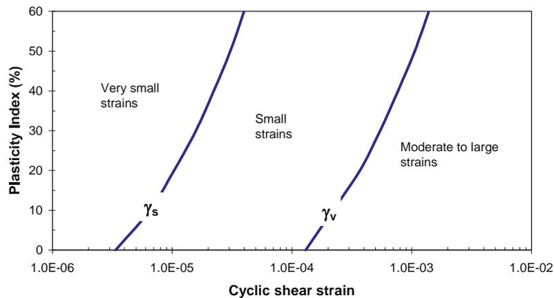
**Figure 6.** Threshold values for cyclic shear strains
