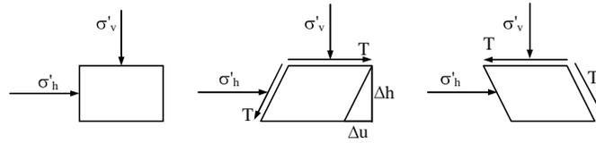
**Figure 2.** Idealized stress cycle during an earthquake
